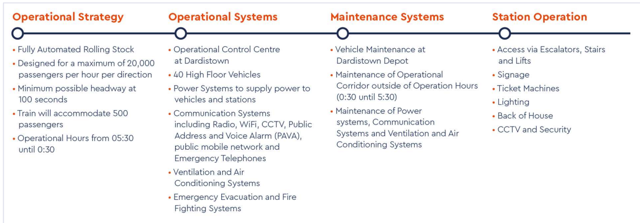
Diagram 1.2: Summary of Key Activities during the Operation Phase of the Proposed Project
